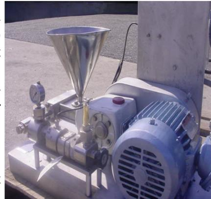
The main advantage is that it has no moving parts. It does not depend upon centrifugal force or mechanical shear. It has good scalability and repeatability. Emulsions made at lower energy consumption than other mixtures that rely on mechanical shear and rotational velocity. Mechanical shear effected by viscosity and volume whereas sonolator is not.
