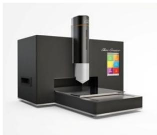
**Nozzle:** The 0.4mm nozzle has an ultra-fine hole that the chocolate come out of, so naturally it is susceptible to blocking if the chocolate has rogue particles or if the room temperate is very low.
